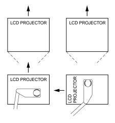
You can project around the projector by moving the arm and the camera head.
